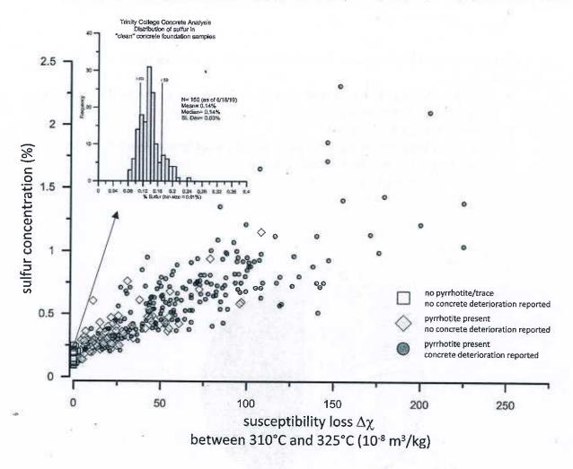
Trinity Concrete Analysis data as of 6/18/19 (from 212 homes, 451 cores). Results are based on two independent, objective tests 1) total sulfur concentration (y-axis) and 2) magnetic susceptibility of pyrrhotite (x-axis).
