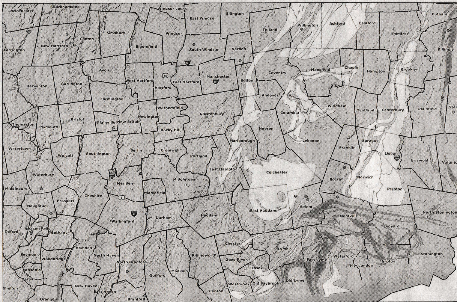
Rocks containing pyrrhotite were found in the areas in white across eastern Connecticut. Rocks containing pyrite were found in the darker gray areas, in the southeast. The dots indicate active quarries in 2014-2015.
